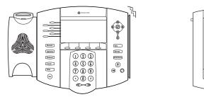
2. Align the Expansion Module at the top of the groove lines on the SoundPoint IP 650 phone and slide unit downwards until unit clicks into position. Connect the Base Stand for each Module.
