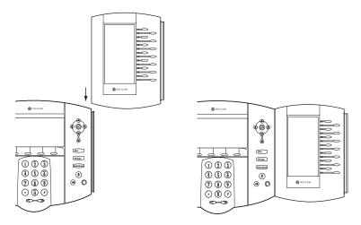
3. To connect up to three Expansion Modules together, repeat steps 1 and 2.
