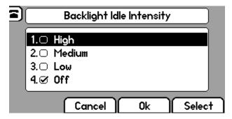
**6.** Use the  $\bigcirc$  or  $\bigcirc$  to select high, medium, low, or off and press the **Select** soft key to modify the Backlight On Intensity.
