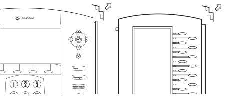
**2.** Align the SoundPoint IP Expansion Module at the top of the groove lines on the SoundPoint IP 650 phone and slide it downwards until it clicks into position.
