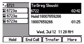
If more than two calls are on hold on a single Line Key, an indication appears on the graphic display, for example "2/3", indicating that this is the second call out of three calls.
