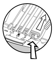
**2.** Align the two protrusions on the bracket with their corresponding holes in the phone.
