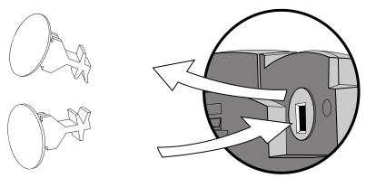
**3.** With mounting tab of the base unit facing up, fasten the base unit to the wall mount using wall anchors (not included).
